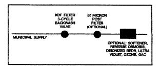
rate to surface of KDF 55 process medium. Inaccurate sizing is the most common reason for trouble in filter systems. The nominal flow rate in the service cycle depends on surface area available. For most types of filter media, the service flow rate must not exceed five gallons per minute (gpm) per square foot of surface area, with at least a 30-inch filter bed depth.
