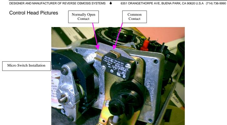
Insert spade connector into open space on connection block. This is the power for the light.
